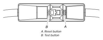
This room air conditioner is equipped with a power supply cord required by UL. This power supply cord contains state-of-the-art electronics that sense leakage current. If the cord is crushed, the electronics detect leakage current and power will be disconnected in a fraction of a second.
